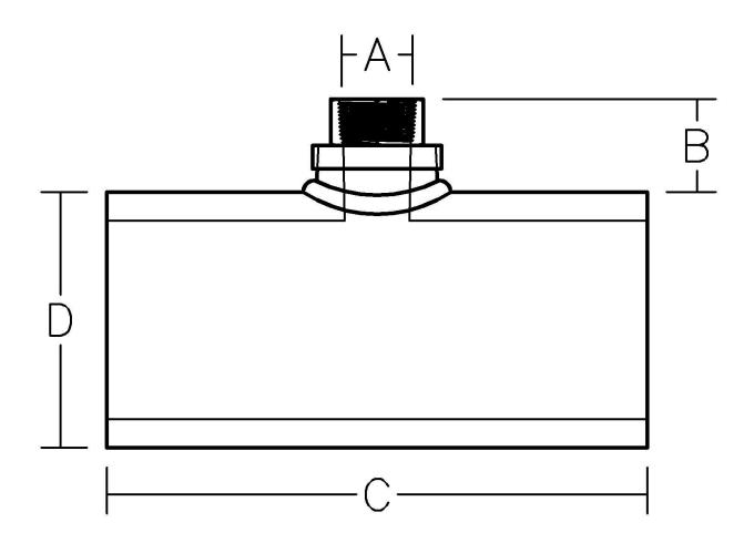
Fully pressure rated • Standard SDR sizes 7,9,11,17 Manufactured to ASTM D3035, D1599, D1598, D3350
